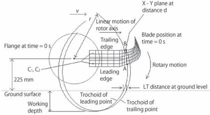
**Fig. 6** Trochoids of leading and trailing points (A and B) of a C-type blade with mounting bolts C<sub>1</sub> and C<sub>2</sub>; velocity ratio 4.97; travel speed (v) 3.50 km/h; angular velocity 23.03 rad/s; rotor speed 220 rpm; blade orientation angle 0 degree; depth 30 mm; rotor radius 210 mm
