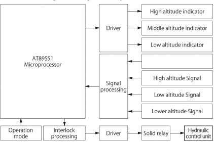
Fig. 3 Block diagram of the hydraulic controller
