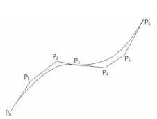
**Fig. 1a** A bezier curve based on seven (6+1) control points
