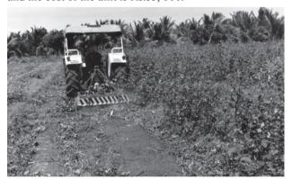
Fig. 1 Tractor operated roto slasher
