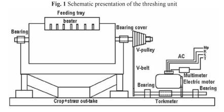
and appropriate specific energy consumption were achieved with pegtooth beater - chromium contrbeater, spike-tooth beater - PVC contrbeater and lama-tooth beater - PVC contrbeater combinations with values of 67.06 %, 0.71 kWh/t, 89.11 %, 0.60 kWh/t, 95.29 % and 0.68 kWh/t for Küsmen, Köylü and Akçin varieties, respectively.
