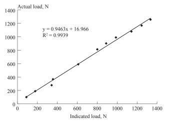
Draft Measurement and Calibration of Dynamometer
