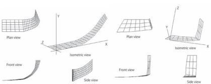
**Fig. 5a** Three-dimensional surface developed for C-type blade
