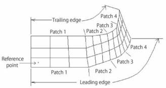
Fig. 4 The complete blade surface generated by joining four patches of control points
