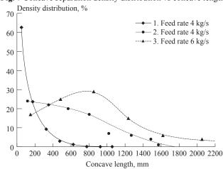
Fig. 7 Concave separation density distribution vs concave length
