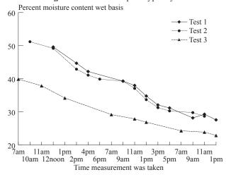
Fig. 10 Rate of moisture loss in production dryer
