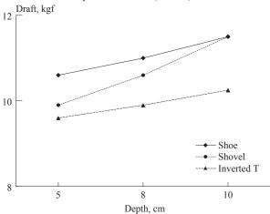
Fig. 7 Relationship between depth of furrow opener and draft (Rabi)
