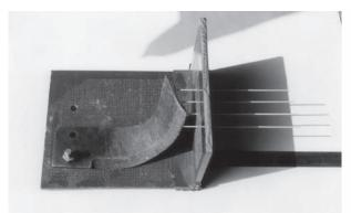
Fig. 3 Schematic setup for measurement of blade coordinates
