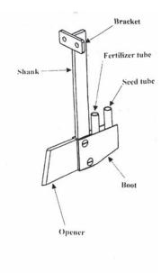
Fig. 2 Development of inverted - T type furrow opener
