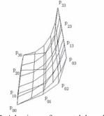
**Fig. 1b** A bezier surface patch based on 4x4 (3+1)x(3+1) control points
