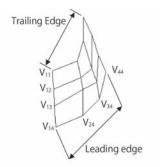
Fig. 2 Control points of developed blade at zero degree orientation in single patch (GS methods)
