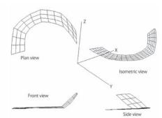
**Fig. 5c** Three-dimensional surface developed for Japanese C-type blade
