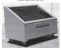
Fig. 2 Photograph of prototype solar cabinet dryer (open)
