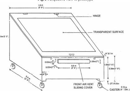
Fig. 3 Perspective view of prototype
