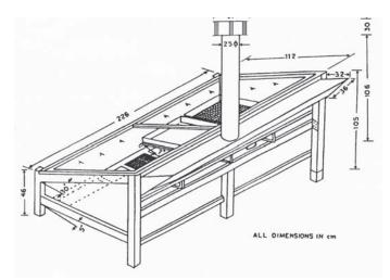
Fig. 3 Solar cabinet dryer with solar-cum-wind aspirator, CIAE, Bhopal
