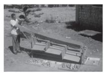
Fig. 2 Raw mango grader
