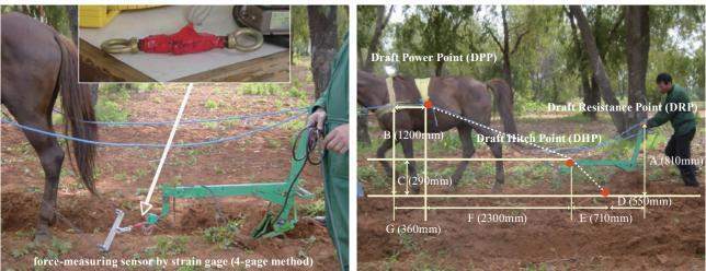
Fig. 1 Experimental devices
