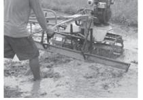
Fig. 8 The spring-activated PhilRice leveler
