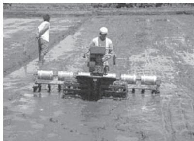
**Fig. 13** The improved hand tractor-drawn paddy seeder
