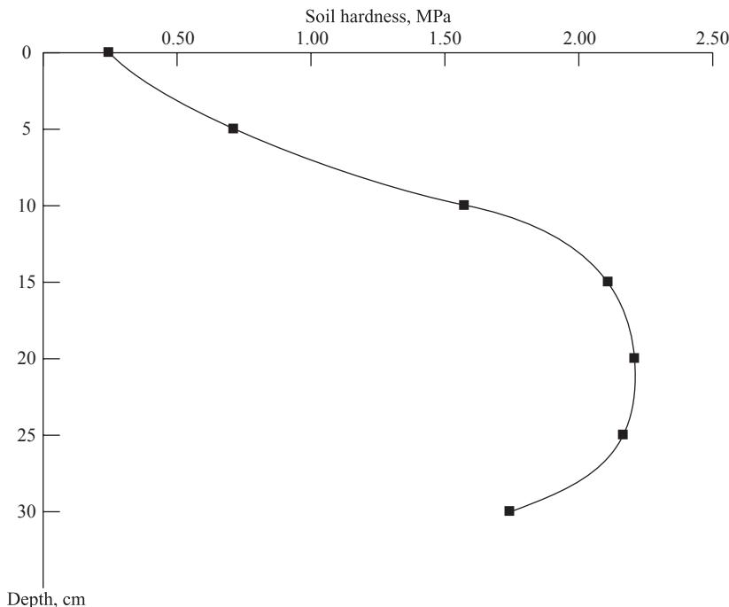
**Fig. 6** Relation between depth (cm) and soil hardness (MPa) as measured by a soil cone penetrometer
