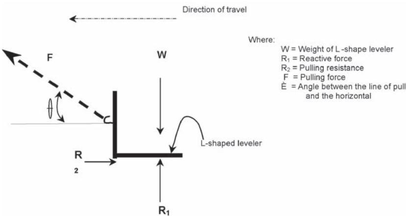
Fig. 10 Force diagram of the hand tractor-drawn leveler
