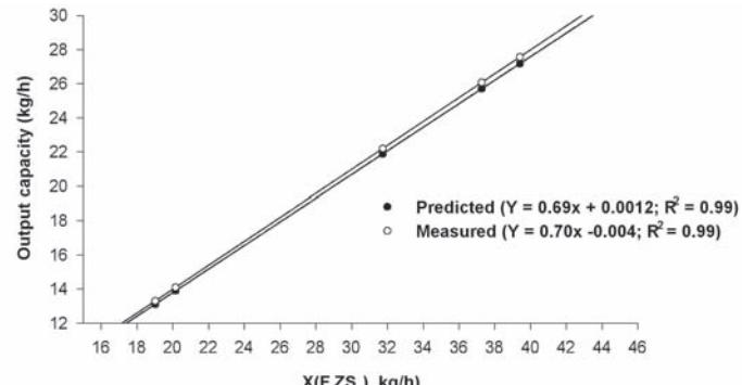
**Fig.6** Output capacity vs product of feedrate, grain-straw ratio and separation efficiency
