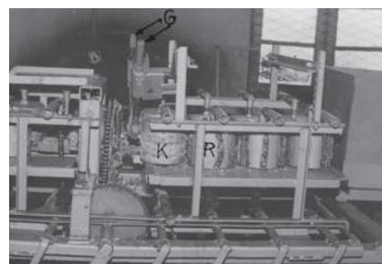
**Fig. 2** The yam peeler showing the rollers, R, K, and tuber guide, G
