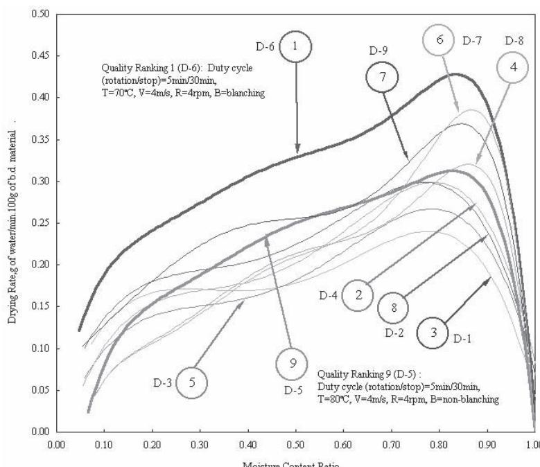
**Fig. 2** Drying rates of the dehydration process of chili pepper
