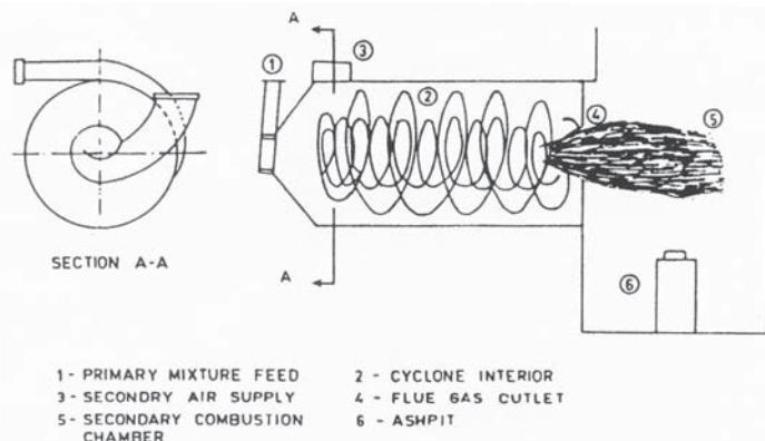
**Fig. 2b** Horizontal cyclone type furnace, IIT, Kharagpur
