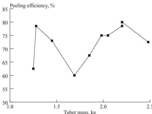
**Fig. 9** Peeling efficiency vs tuber mass
