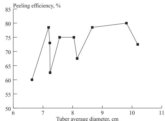
Fig. 8 Peeling efficiency vs tuber average diameter
