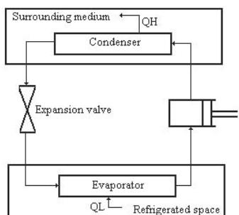
Fig. 2 Basic components of a refrigeration system and typical operating conditions
