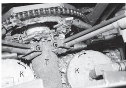
**Fig. 4** Tuber, T, being fed to the peeling chamber. K - Spiked roller, G - Tuber guide, A-Peeler arm
