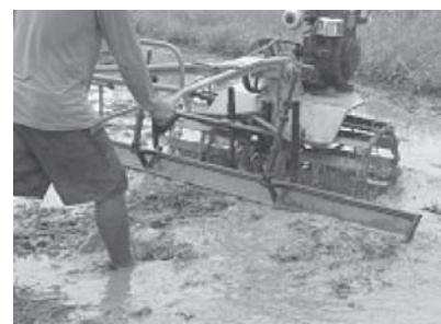
**Fig. 8** The spring-activated PhilRice leveler
