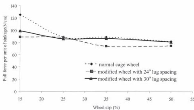
**Fig. 10** Pull force per unit of sinkage (N/cm) at different slips for normal and modified wheel
