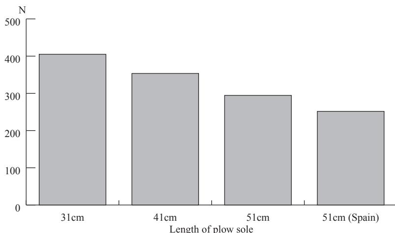
**Fig. 11** Comparison of the standard deviation (SD) values for plow draft-force data for plows with various sole lengths
