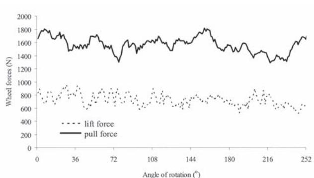
**Fig. 4** Forces on the cage wheel with opposing lugs at 15° circumferential angle, 30° lug angle, 24° lug spacing at 25 % slip
