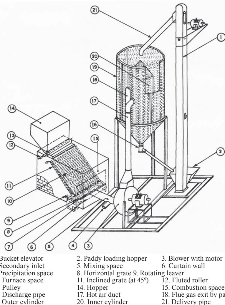
**Fig. 6** Pictorial view of recirculating batch dryer coupled with rice husk fired furnace for paddy drying developed at IIT, Kharagpur
