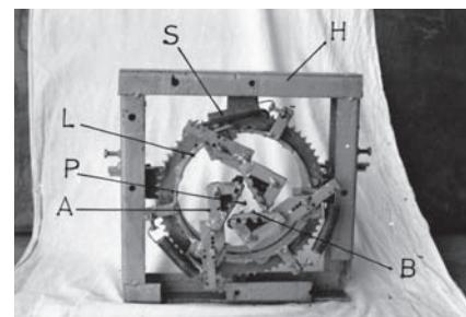
**Fig. 3** The peeling chamber. A - Peeler arm, B - Peeler blade, H - Peeler ring housing, S - Spring, L - Peeler ling
