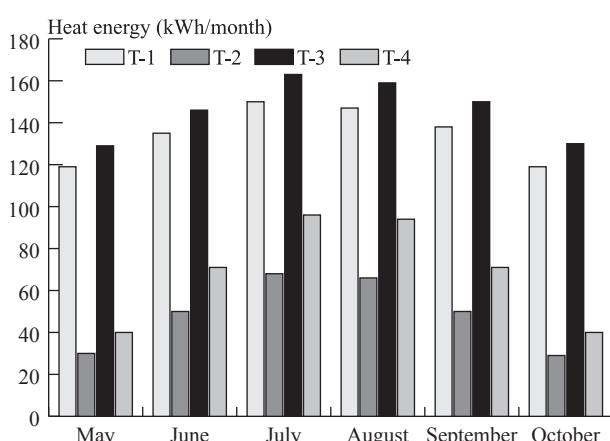
Fig. 5 The heat energy given to the ambient air by the condensers of the coolers
