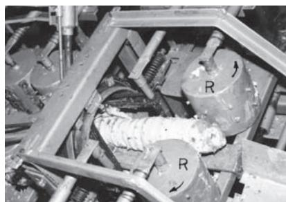
**Fig. 5** Peeling operation about to be completed. R - Lager withdrawal roller
