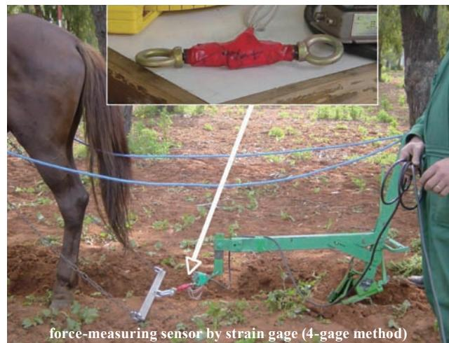
Fig. 1 Experimental devices
