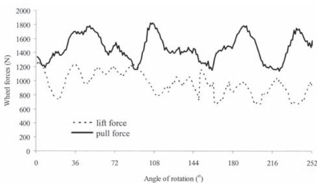
**Fig. 5** Forces on the cage wheel with opposing lugs at 15° circumferential angle, 30° lug angle, 30° lug spacing at 25 % slip
