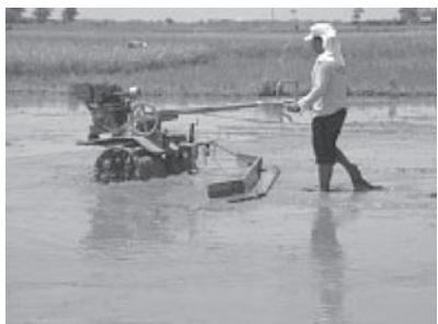
**Fig. 9** The prototype L-shaped drag-type leveler
