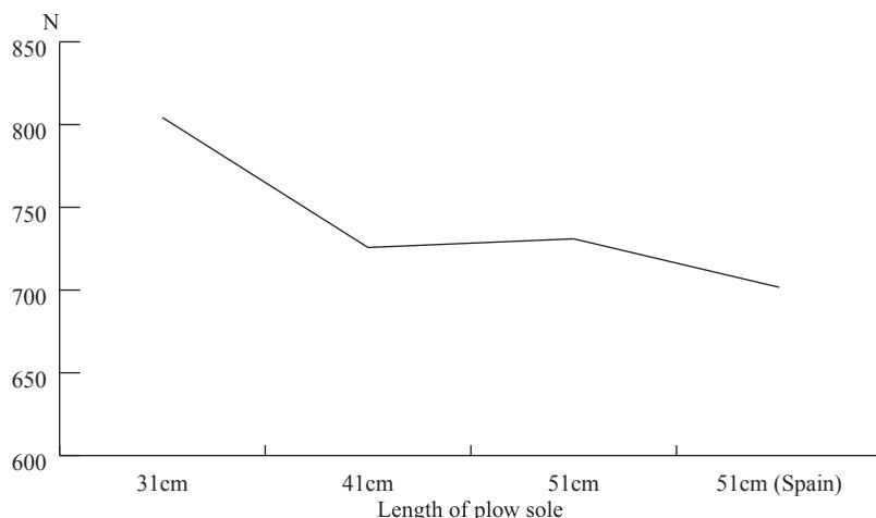
**Fig. 9** Average plow draft force with different plow sole length
