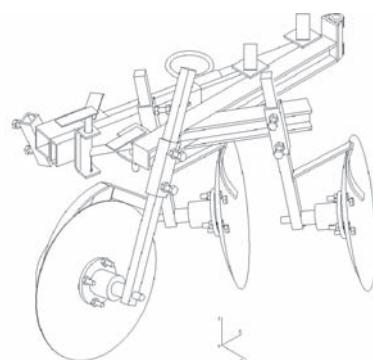
**Fig. 5** Disc plow configured for normal plowing
