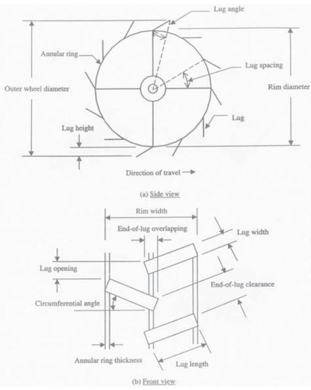
Fig. 2 Sketch of cage wheel parameter, (a) side view; (b) front view (Watyotha and Salokhe, 2001)
