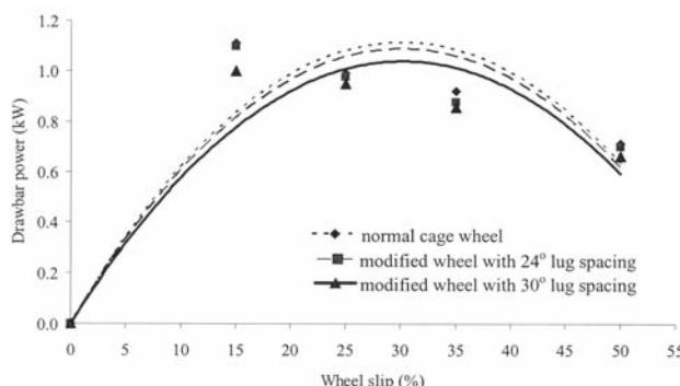
**Fig. 12** Drawbar power of normal cage wheel and cage wheel with opposing circumferential lugs (modified wheel) at various slips
