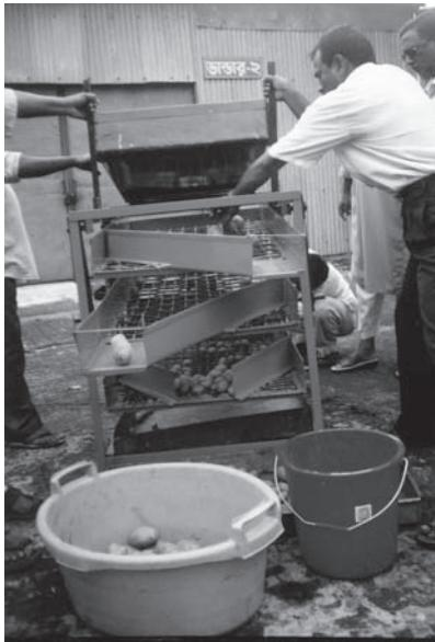
**Fig. 2** Potato grader in operation
