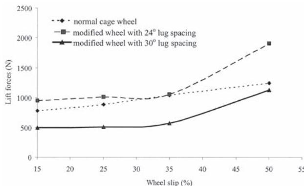
**Fig. 7** Variation of lift forces at different slips for normal cage wheel and cage wheel with opposing circumferential lugs  $24^\circ$  and  $30^\circ$  lug spacing
