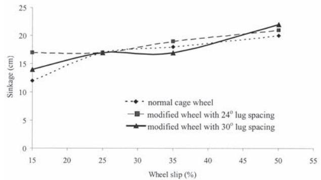
**Fig. 9** Sinkage variation (cm) at different slips for normal and modified wheel
