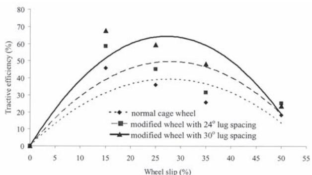
**Fig. 13** Tractive efficiency of normal cage wheel and cage wheel with opposing circumferential lugs (modified wheel) at various slips
