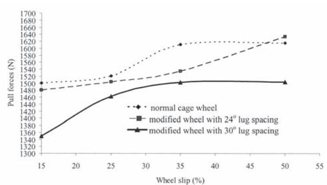
**Fig. 6** Variation of pull forces at different slips for normal cage wheel and cage wheel with opposing circumferential lugs 24° and 30° lug spacing
