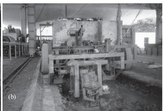
**Fig. 8** Soil track on lugs of (a) normal wheel and (b) modified wheel at slip 50 %
