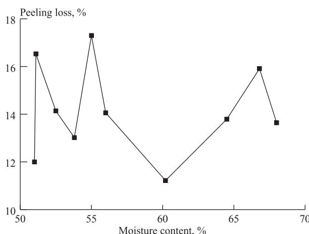
**Fig. 11** Peeling loss vs tuber moisture content
