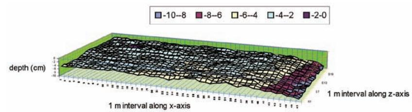
Fig. 12 Field surface profile after leveling
