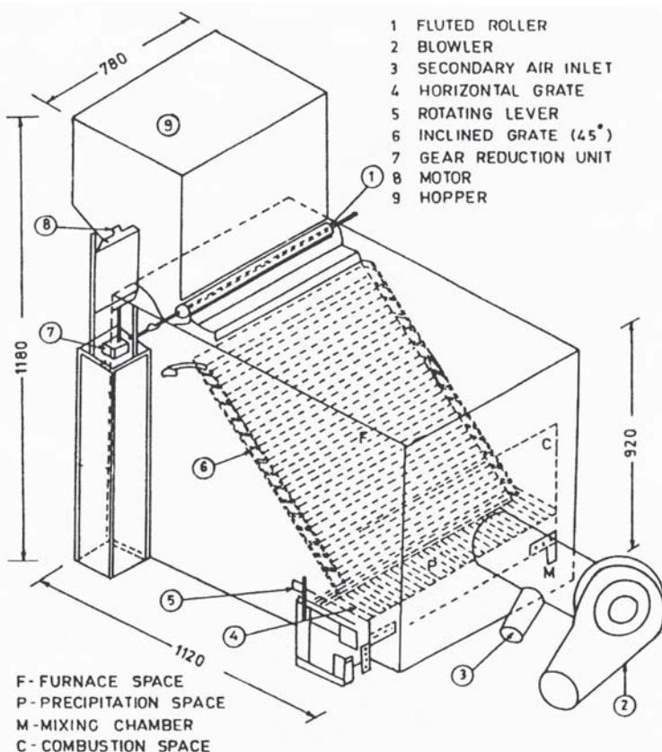
Fig. 1 Box type inclined grate paddy husk fired furnace developed at IIT, Kharagpur
