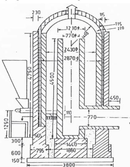
**Fig. 2a** Vertical cyclone type husk fired furnace, FCI, Thanjavur
