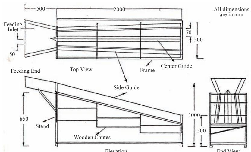
**Fig. 1** Raw mango grader
