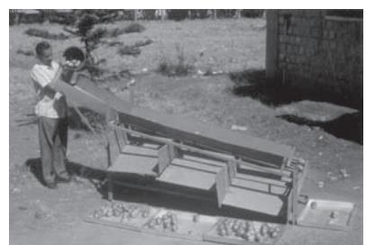
**Fig. 2** Raw mango grader
