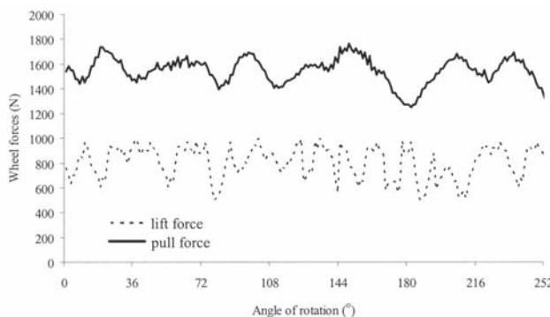
**Fig. 3** Forces on the nomal cage wheel at 30° lug angle, 30° lug spacing at 25 % slip
