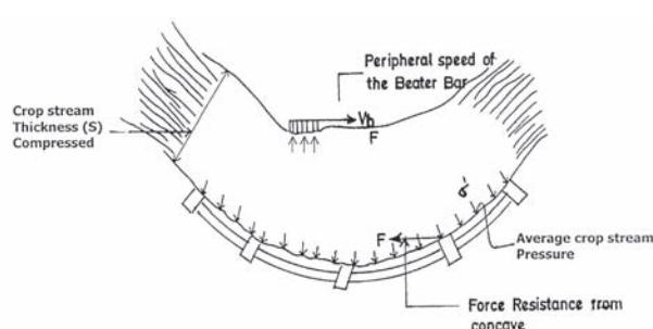
**Fig.3** Force analysis of the crop stream in the threshing zone
