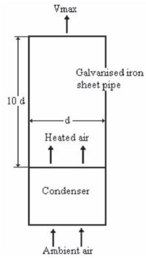
**Fig. 4** Connection of the galvanized iron sheet pipe to the condenser
