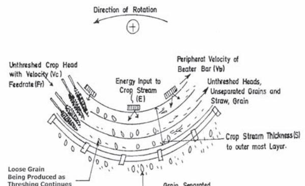
**Fig. 2** Schematic description of crop motion during threshing and separation processes of the model
