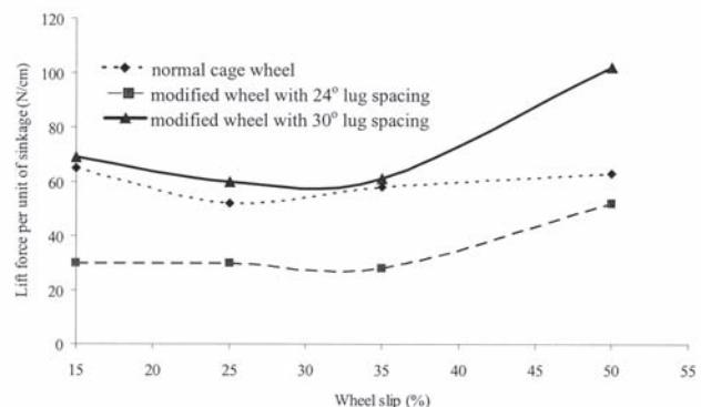
**Fig. 11** Lift force per unit of sinkage (N/cm) at different slips for normal and modified wheel
