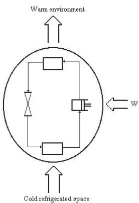
Fig. 1 Schematic presentation of the coolers
