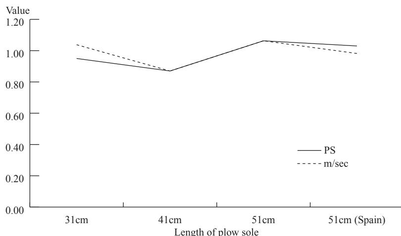
**Fig. 10** Required horse power (PS) and speed during plowing
