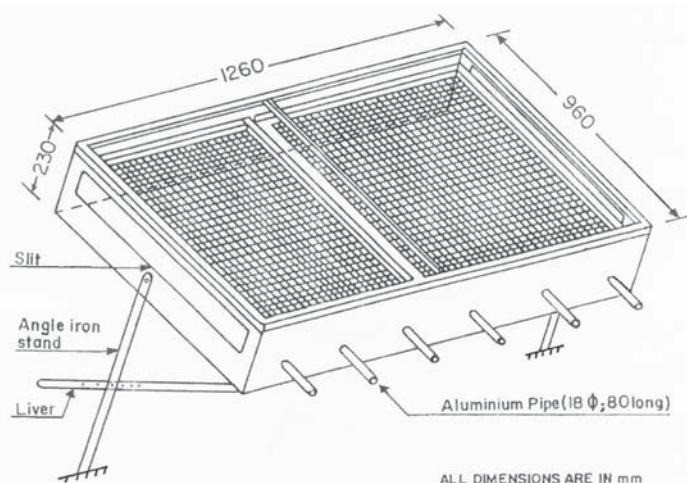
**Fig. 5** Inclined direct type natural convection solar dryer developed at CAZRI, Jodhpur
