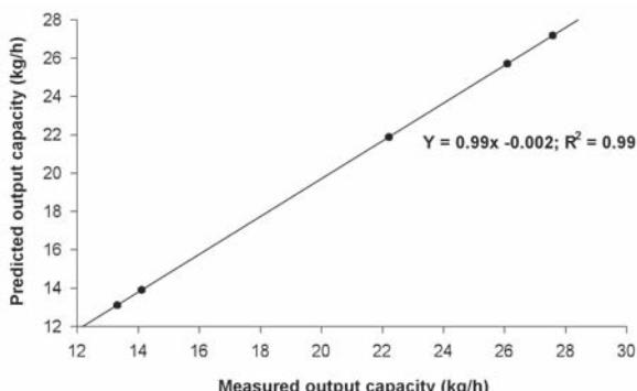
**Fig.5** Mesured vs predicted capacity for a millet thresher
