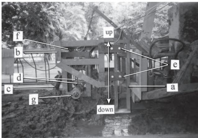
Fig. 1 Cage wheel test facility with free sinkage system (a: fixed frame; b: movable frame; c: test wheel; d: sprocket and chain; e: roller bearing; f: octagonal ring transducer; g: slip ring)
