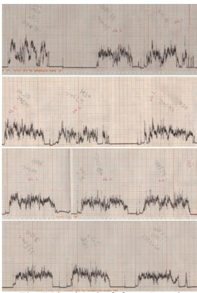
**Fig. 7** Plowing draft force (actual measurement curves)
