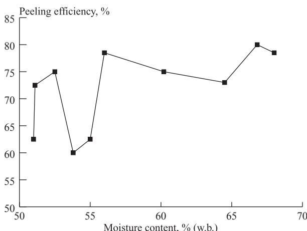
Fig. 7 Peeling efficiency vs tuber moisture content
