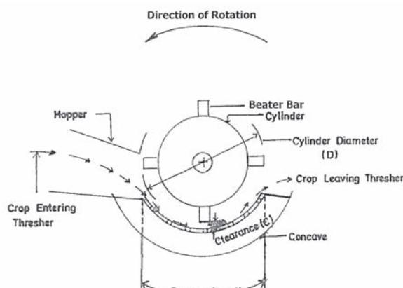
**Fig. 1** Cylinder-Concave arrangement of the spike tooth thresher
