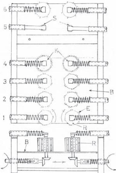
**Fig. 1** Diagrammatic view of the conveyor system
