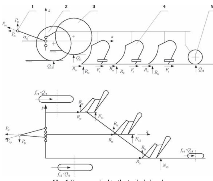
Fig. 1 Forces applied to the trailed plough
