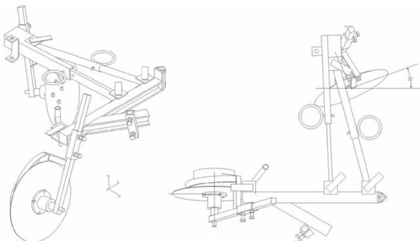
**Fig. 4** Disc plow configured for levee side plowing
