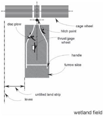
**Fig. 2** Schematic diagram showing the untilled land strip along the side of the levee
