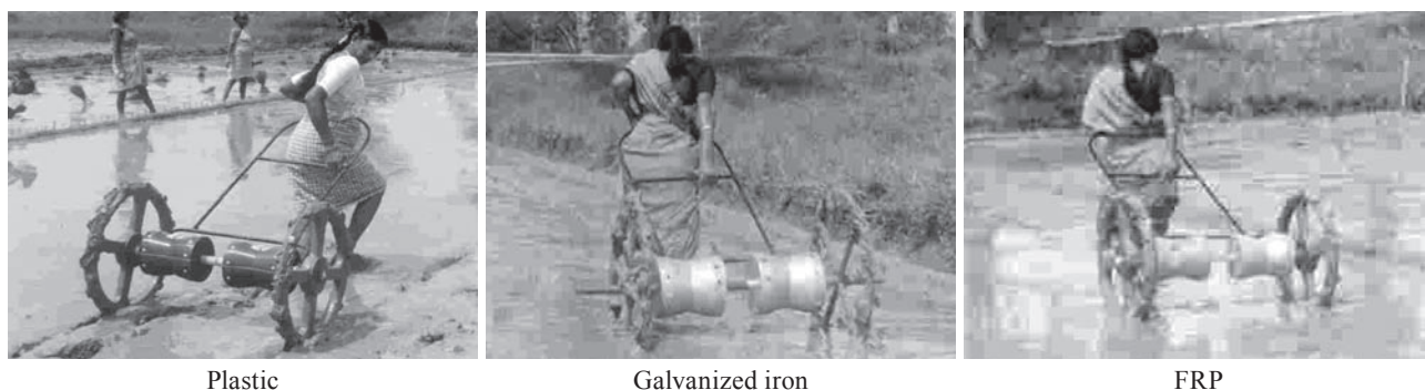
Fig. 2 Four row paddy seeder in operation
