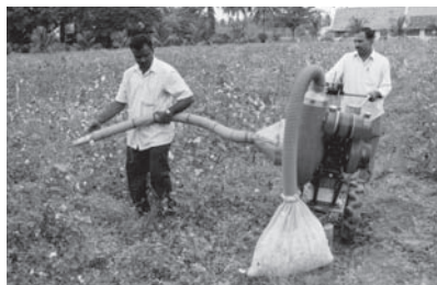
Fig. 2 Engine operated pneumatic cotton picker in field operation
