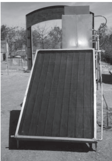
Plate 1 Solar geyser cum distillation unit
