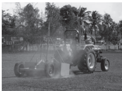
Fig. 5 Operational view of laser leveler
