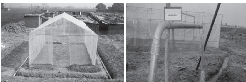
Fig. 2 Pictorial view of greenhouse integrated to aquifer water thermal control system
