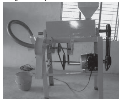
Fig. 3 Chickpea dehuller - front view
