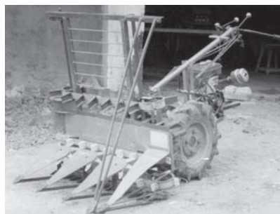
Plate 1 Improved self propelled vertical conveyer reaper machine for cereals and tall fodder crops
