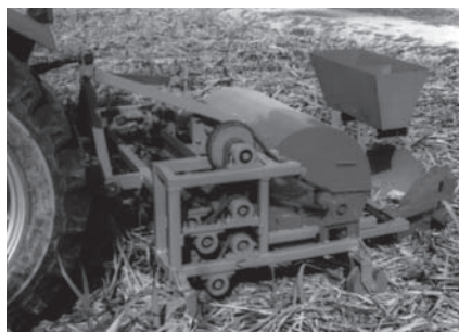
Fig. 5 IISR trash handling equipment
