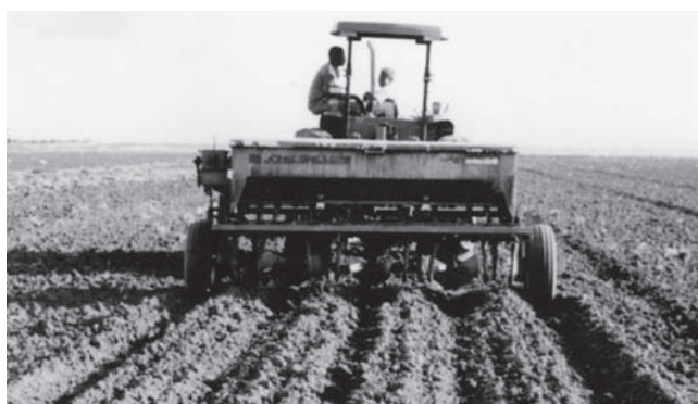
Fig. 1 The modified bed planter rear view during field testing in the first season
