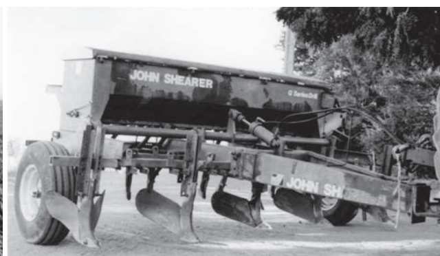
Fig. 2 Front view of the modified bed planter
