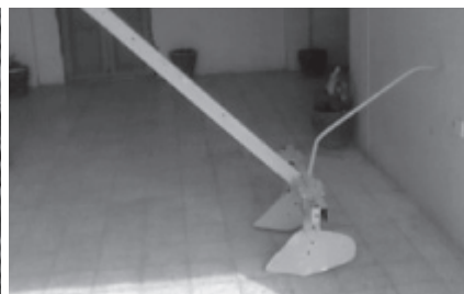
Fig. 1b The second design of the HAFEED ridger (side view)
