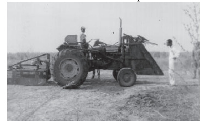
Fig. 7 Tractor operated sugarcane harvester coupled to the tractor in readiness for field operation
