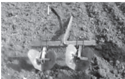
Fig. 1a The second design of the HAFEED ridger (rear view)
