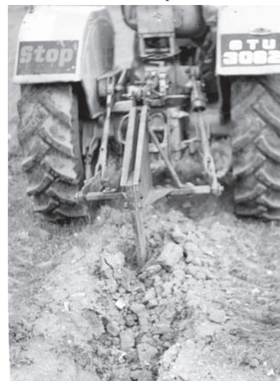
Fig. 2 Tractor drawn conventional subsoiler in operation
