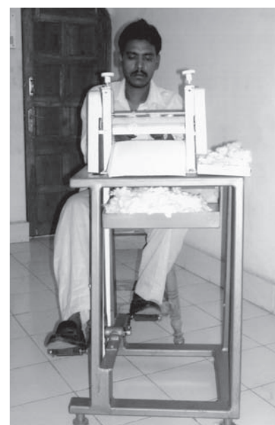
Fig. 5 Foot operated gin in operation
