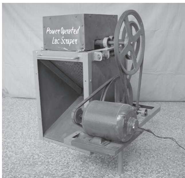
Fig. 1 Power operated roller type lac scraper
