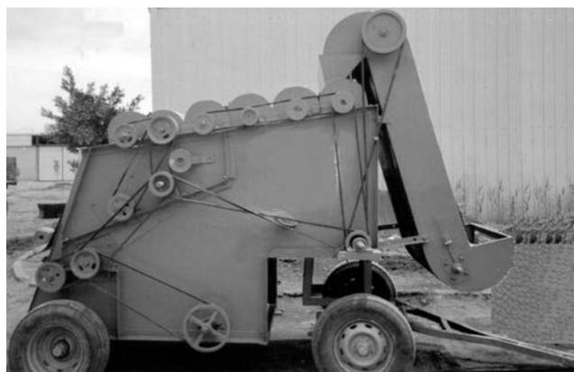
1. Mechanical loader, 2. Chain conveyer, 3. Strip, 4. Tank, 5. Feeder roller, 6. Impact drum, 7. Concave, 8. Saw drum, 9. Doffing drum, 10. Trash auger, 11. Division, 12. Inclined surface, 13. Frame body, 14. Wheels, 15. Hitch point, 16. Revolving circle
