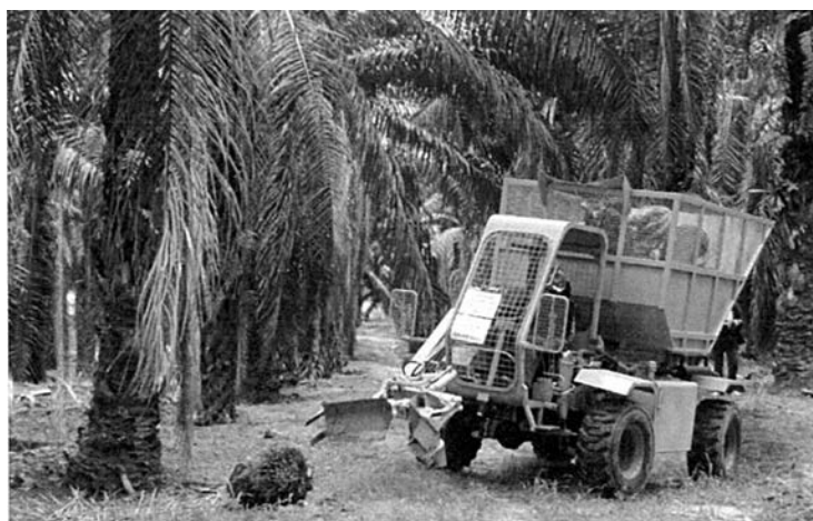
Fig. 2 The developed prototype of new machine system for in-field FFB collection-transportation operation
