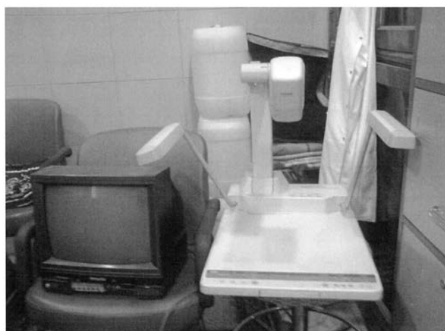
b) A vision apparatus for color analysis.
