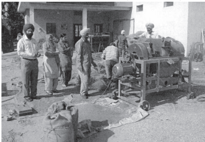
Fig. 2 Modified spike-tooth thresher being used for threshing lentil
