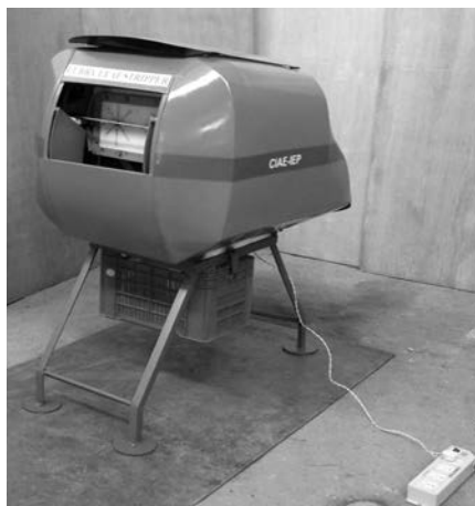
Fig. 4 Power operated curry leaf stripper
