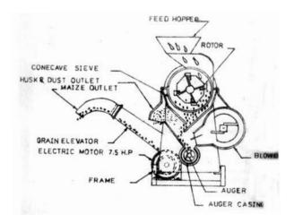
Fig 6 Pedal operated Maize Dehusker-sheller (MPUAT, Udaipur)
