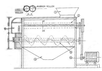
Fig 7 TNAU Maize Dehusker-sheller
