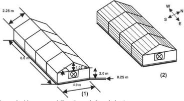
1. Covered with corrugated fiberglass reinforced plastic,
