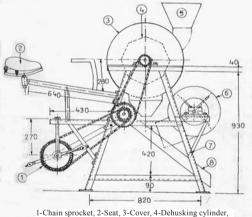
1-Chain sprocket, 2-Seat, 3-Cover, 4-Dehusking cylinder, 5-Hopper, 6-Blower, 7-Stand/Frame, 8-Tray
