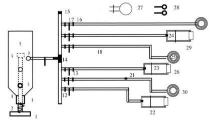
1- Handle, 2- Spring, 3- Axle, 4- Fixed nut. 5- Tank, 6- Fuel hole, 7-Manometer, 8- Bluff., 9- Out put hole, 10- Main value, 11- Distributor, 12- Copper socket, 13- Plug, 14- Tees, 15- Reserve socket, 16- Clips, 17- Kerosene regulator value, 18- Rubber hose with thermal wire, 19- Pipe, 20- Elbow, 21- Socket, 22- out chamber, 23- Evaporate pipe, 24- Nozzle, 25- inside chamber, 26- Throat, 27- Fixed tin, 28- Fixed screws, 29- Upper blowpipe, 30- Lower blowpipe.
