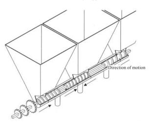
Fig. 1 Fertilizing hoppers
