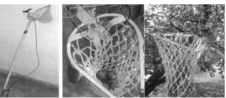
A fruit picker of adjustable height was developed to overcome human drudgery by traditional fruit picking practice. Although the device is simple in design, yet very effective. The device consisted of Clutch lever, a clutch wire, an extension mechanism, a cutting mechanism and head with a flexible basket for fruit collection. It can pick fruits up to a height of 5-6 meter and weighs only
