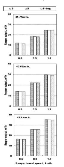
from 2 to 8°. At 35.7 % w.b. and 5°, field efficiency increased from 58.14 to 63.11 % (+8.55 %) by increasing reaper travel speed from 0.6 to 1.2 km/h. The highest value of 84.89 % field efficiency was obtained at 45.4 % w.b., 1.2 km/h and 2°. The lowest value of 55.16 % was obtained at 35.7 % w.b., 0.6 km/h and 8°. The difference between the highest and lowest values of field efficiency could be estimated at 53.9 %.
