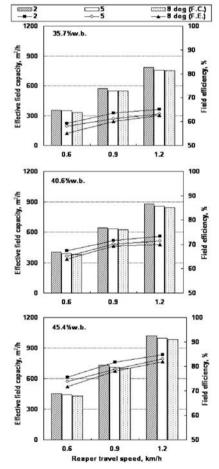
h (+100 %). The highest value of 1,018.68 m<sup>2</sup>/h effective field capacity was obtained at 45.4 % w.b. litter moisture content, 1.2 km/h reaper travel speed and 2° shovel blade tilt angle. The lowest value of 330.96 m<sup>2</sup>/h was obtained at 35.7 % w.b., 0.6 km/h and 8°. The difference between the highest and lowest values of effective field capacity could be estimated at 207.8 % increment.
