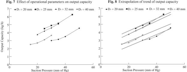
Fig. 8 Extrapolation of trend of output capacity
