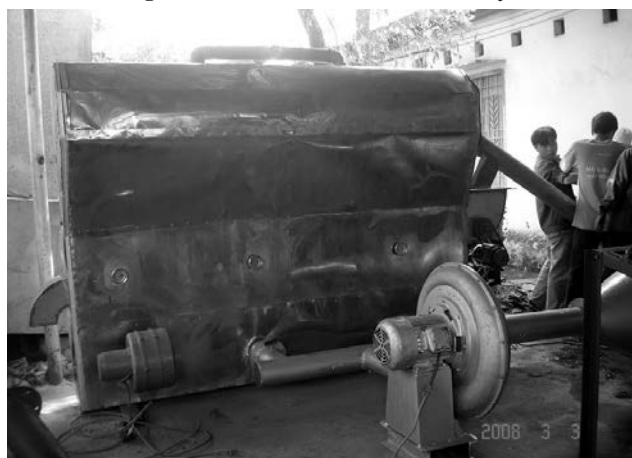
Fig. 2 The fabricated fluidized-bed dryer
