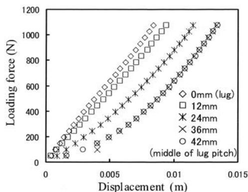
**Fig. 3** Approximation of the interactive relationships between the rubber crawler and the loading force acting on the track roller
