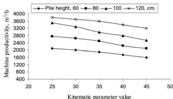
Fig. 4 Effect of kinematic parameter value on composting density at different pile heights
