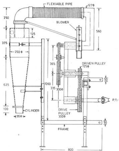
**Fig. 6** Front elevation of experimental picking aid (all dimensions are in mm)
