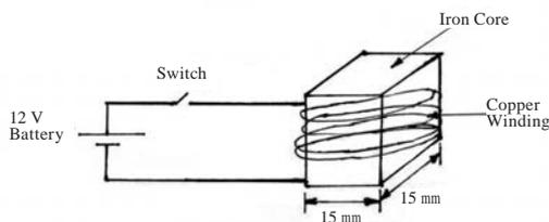
**Fig. 3b** A View of coil arrangement in mechanical valve
