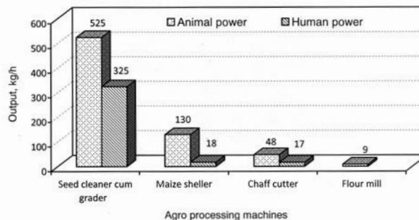
it reduced the drudgery and labour cost. The shelling efficiency of the maize sheller was 93 percent. The chaff cutter operated by the animal powered gear gave about 3-4 times more output as compared to hand operated chaff cutter. Further, there was an erratic supply of electrical power in rural areas, which supports the suitability of animal-based rotary mode complex.
