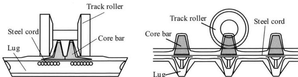
**Fig. 2** The vertical load forces acting on a track roller and the vertical displacements of the rubber crawler
