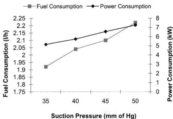
**Fig. 8** Effect of suction pressure on power and fuel consumption for open valve
