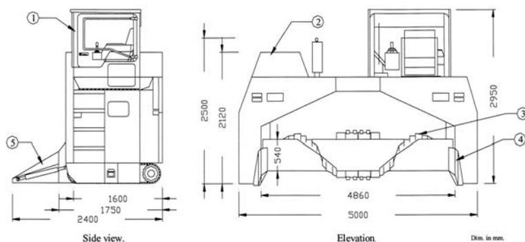
1 Cabaine 2 D. engine 3 Turning knives 4 Turning drum 5 Heap opener
