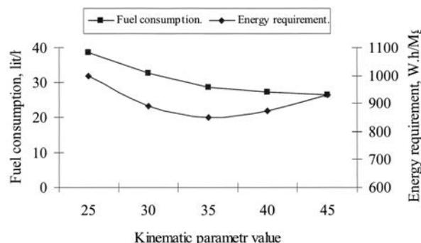
**Fig. 6** Effect of kinematic parameter value on hourly and turning cost at different pile heights
