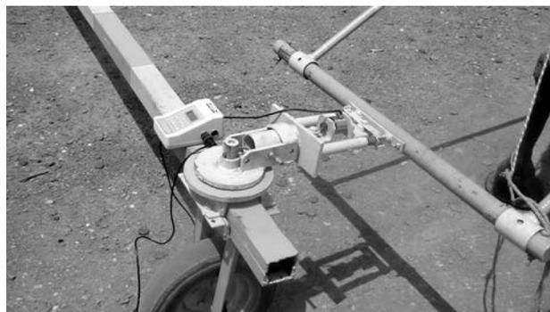
**Fig. 5** Testing of power transmission unit by animal loading car
