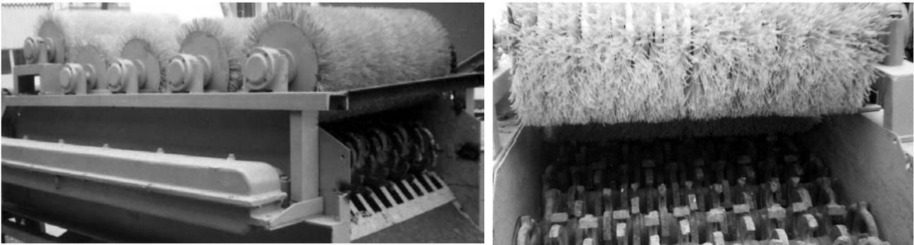
Fig. 3 Schematic view of the Armer Salmon Hippo beet cleaning machine
