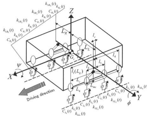
Fig. 5 The dynamic spring constants and viscous damping coefficients of the rubber crawler
