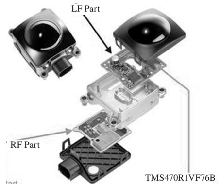
Bosch LRR2 with dimensions of 73 × 70 × 60 mm (2.9 × 2.8 × 2.4 in) can be integrated almost anywhere on the front of the vehicle
