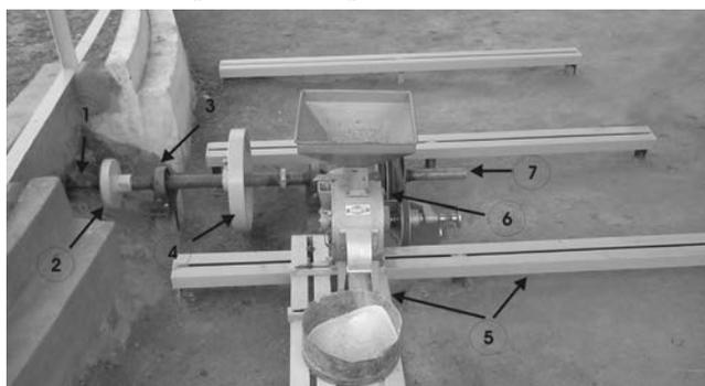
**Fig. 4** Hitching arrangement and measurement of pull
