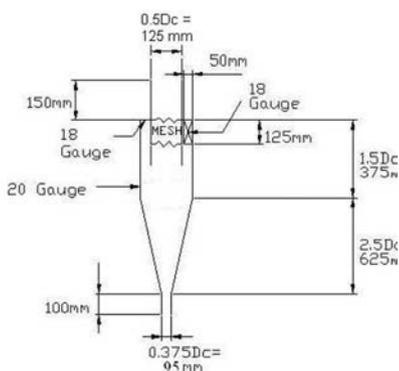
Fig. 2 Various sections causing pressure losses
