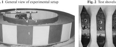
1. Soil bin 2. Horizontal beam 3. Worm gear unit 4. DC motor 5. Pneumatic wheel 6. Tool frame 7. Shovel
