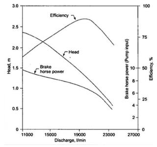
Fig. 9 Performance curves of a typical propeller pump
