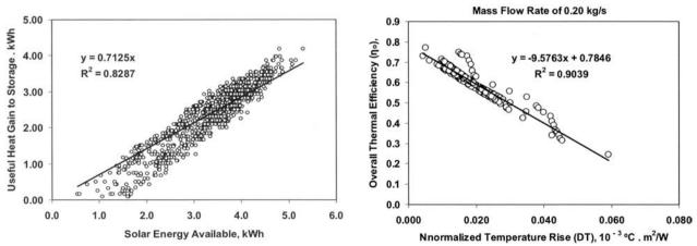
Fig. 4 Solar energy collected (useful to storage) versus solar energy available during the experimental period
