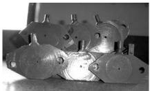
The equipment studies were conducted to determine the injection rate through the different sizes of the orifice meters. After preparing the fertilizer solution, the water flowing through orifice meter was applied to the area under fertigation. All developed equipment were tested under various inlet discharges and rates of fertilizer injection. All orifice meters were tested for areas  $450 \text{ m}^2$ ,  $300 \text{ m}^2$  and  $150 \text{ m}^2$
