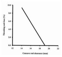
Fig. 8 Effect of side concave clearance on threshing unit loss
