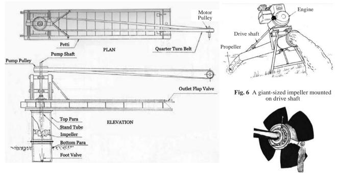
can be used as portable units operated by light weight engines or in permanent installations using electric motor or engines. Propeller pumps are axial flow pumps in which the pressure head is developed mostly by the propelling or lifting action of the propeller blades on water. It can be used as portable units operated by light weight engines or in permanent installations using electric motor or engines.
