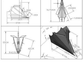
Fig. 2 Isometric and orthographic diagram of raised bed seed cum fertilizer drill
