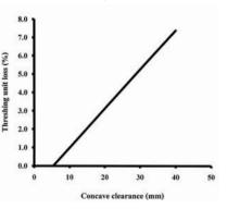
Fig. 6 Effect of concave rod clearance on threshing unit loss
