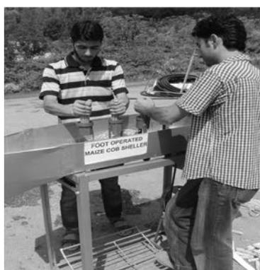
**Fig. 4** Horizontal maize cob sheller in operation
