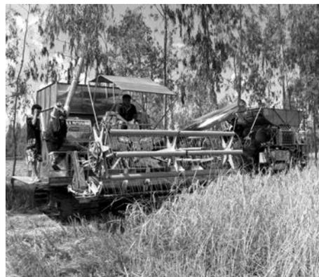
**Fig. 2** Axial flow threshing unit
