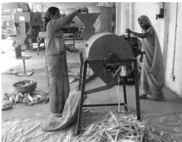
Fig. 1 Farm woman operating the 1st prototype of hand operated maize dehusker-sheller
