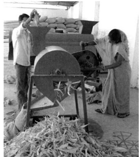
Fig. 5 Farm woman operating the final prototype of hand operated maize dehusker-sheller
