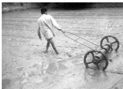
Fig. 1 A view of Improved Direct Paddy Seeder in working condition
