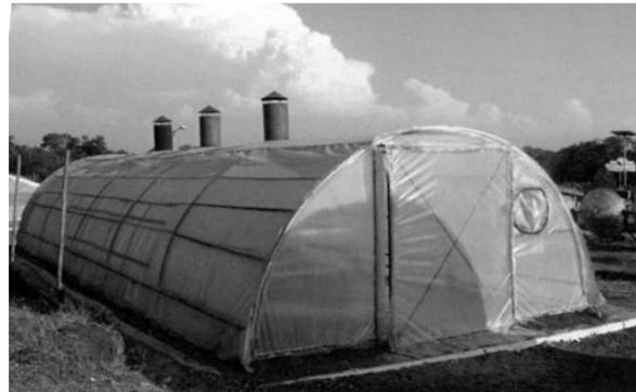
**Table 3** Technical specifications of solar tunnel dryer for fish (100 kg/ batch)
