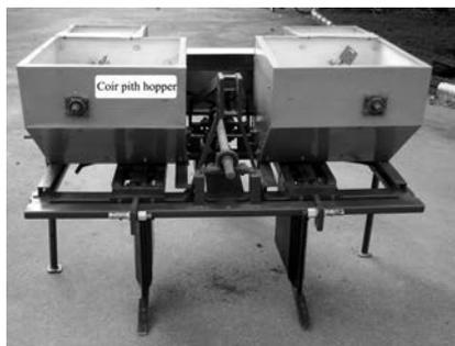
**Fig. 2** Two row subsoil organic mulch cum fertilizer applicator (side view)
