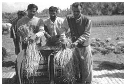
Fig. 3 Motor operated paddy thresher
