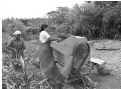
**Fig. 5** Operational view of arecanut stripper with men workers
